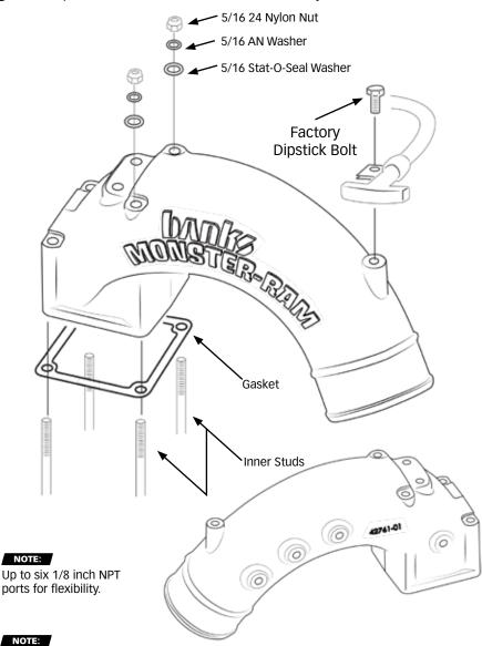
The 1/8" NPT ports shall only be used for installing sensors for measuring air temperature, pressure, or flow. Sensors installed to these ports shall have a fitting of 1/8" NPT and shall not be connected to the vehicle's electronic control units. In addition, factory sensors that come equipped on the vehicle shall not be disconnected and shall not be relocated to the ports. The ports, when not used, shall be closed off with the supplied plugs.
