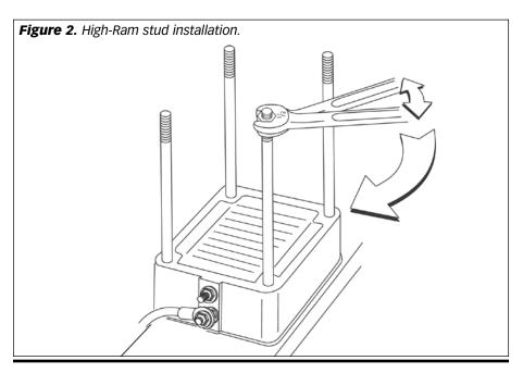
**13.** CAUTION: The High-Ram/ Monster-Ram studs have different threads on each end. Make sure the M8 ends go into the engine intake manifold. The shorter studs are placed inboard closest to the valve cover. Apply blue medium strength thread locking compound to the M8 threaded end of the studs. Hand tighten the studs to the intake manifold.
