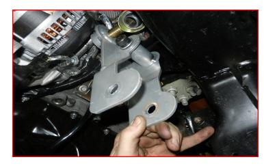
Install the ReadyLift passenger side differential drop into the factory location using factory hardware. Do not tighten at this time.
