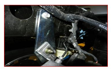
Install the rear emergency brake line drop bracket to the frame using the factory hardware, the emergency brake line bracket to the drop bracket using 5/16" x 1" bolt, washers and lock nut. Torque to 10 ft-lbs.
