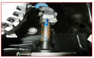
Disconnect the electrical leads to the rack and pinion. Support the rack and pinion and remove hardware from the frame. Carefully lower the rack & pinion assembly from the vehicle and set aside.
