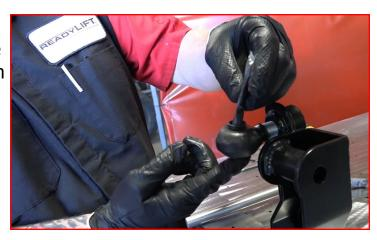
Install the driver side drop bracket into the factory location using the 14mm x 90mm Allen bolt and flat washer. Do not tighten at this time.
