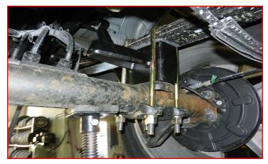
Install the rear brake line drop bracket to the frame using factory hardware. Gently pull the rear hard lines down and attach the rear brake line bracket to the drop bracket using 5/16" x 1" bolt, washers, and lock nut. Torque all to 10 ft-lbs.
