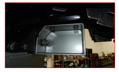
Install the ReadyLift rear cross member into the factory control arm frame pockets using M18 x 150mm bolts, flat washers, and lock nuts.
