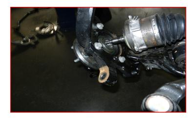
Take vacuum actuator and move to knuckle mounting surface making sure to engage the splined inner ring to the hub assembly and that the vacuum ports are pointing to the top of the knuckle. Install vacuum actuator using factory hardware. Torque to 132 in-lbs.
