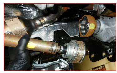
Remove both the driver side and passenger side CV axle. Strike the shaft with a mallet or soft hammer to dislodge it from the c-clip. Support the differential with a suitable jack. Remove the vent tube. Remove the 3 differential mounting bolts from the frame and lower the differential out of vehicle. Diesel models will need to skip to the cutting of the driver side control arm pocket before removal then come back to these steps.
