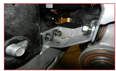
Install rear differential mount using 9/16" x 4" bolt, flat washers, and lock nut. Do not tighten at this time.
