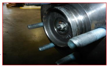
Install dust shield to knuckle using factory hardware. Torque to 5 ft-lbs. Install rotor and brake caliper assembly to hub assembly and knuckle using factory hardware. Apply a drop of thread locker to threads and torque to 148 ft-lbs.
