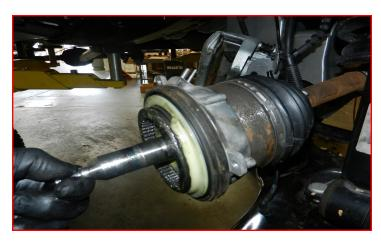
Install the ReadyLift knuckles onto the lower ball joints using factory ball joint nut, 3/4" washer. Run tight at this time. Will torque in later step.
