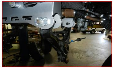
Tighten all differential, rack and pinion, and cross member hardware at this time. Starting with differential, torque all differential hardware to 95 ft-lbs, differential brace to cross member to 45 ft-lbs, cross member main hardware to 200 ft-lbs, sway bar drop bracket hardware to 60 ft-lbs, rack and pinion to front cross member hardware to 150 ft-lbs.
