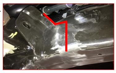
If your differential has the front assembly tab in the middle of the assembly, mark a straight line even with the housing and using a suitable cutting device, remove.
