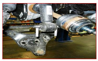
Remove the strut from the frame.
