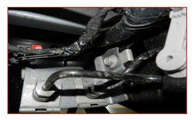
Slightly loosen but do not remove the driver side u-bolts. Remove the passenger side u-bolts completely. Lower the axle just enough to remove the factory block and install the lift block.
