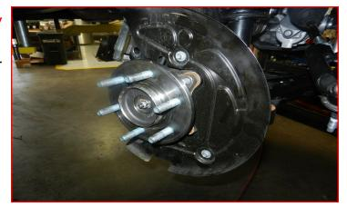
Install the factory brake line bracket to knuckle using 6mm bolt, and washer. Install ABS wire to knuckle using factory hardware. Torque all 5 ft-lbs. Install vacuum lines to vacuum actuator.
