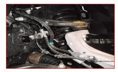
Disconnect the vacuum line from the actuator on the backside of the knuckle.
