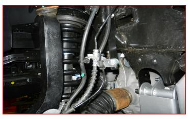
Install outer tie rod ends to knuckle using factory hardware. Torque tie rod end nut and lower ball joint nut to 110 ft-lbs. Install sway bar to drop brackets using factory hardware. Torque to 35 ft-lbs. Install end links to lower control arm using factory hardware. Torque to 40 ft-lbs. Install the wheels and tires and lower the vehicle to the ground. Torque lug nuts to wheel manufacturer specifications.
