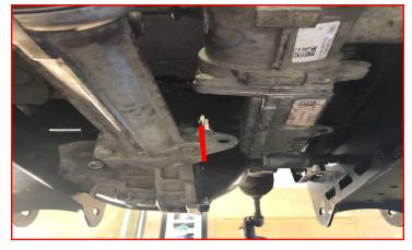
Locate the driver side differential drop bracket and the 3/4" rod end. Install the rod end into the bung on the drop bracket until. Screw into the bung until you measure from the face of the bung to the middle of the heim joint 1.75". The heim joint housing will end up slightly tilted to the back of the truck once installed. Do not tighten the set screw at this time.
