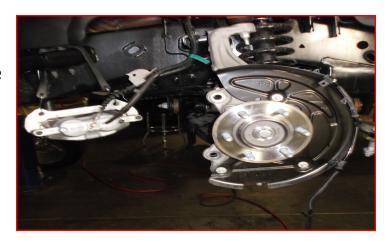
Loosen the upper ball joint nut. Strike the ball joint boss on the knuckle with a dead blow hammer to dislodge the taper.
