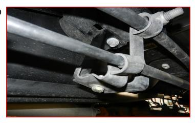
Install new rear shocks with factory hardware. If installing the kit black shocks, the body goes to the ground the same as the factory. If installing other shocks, refer to their directions for install. Do not tighten at this time.
