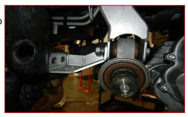
Install the ReadyLift sway bar brackets to corresponding sides of the frame using 7/16" x 1 1/4" bolts, flat washers, and lock nuts. Do not tighten at this time.
