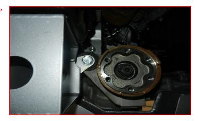
Install the ReadyLift front cross member using the factory hardware from the rear of the vehicle facing forward. Do not tighten at this time.
