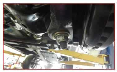
Raise knuckle towards upper control arm while guiding the axle shaft into the hub assembly.
