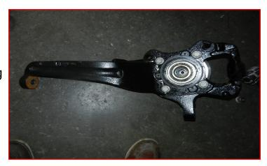
Locate the vacuum hub assembly and place onto the factory axle.
