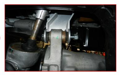
Install the ReadyLift differential brace on the driver side differential drop bracket using 9/16" washer and lock nut. Install the crush tube into the frame using the factory hardware. Do not tighten at this time.
