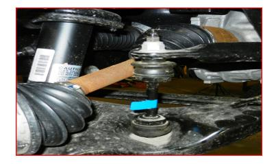
Remove the lower strut mount from the lower control arm.
