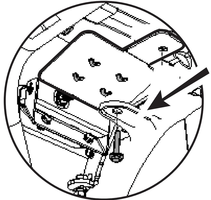
Once the Harness is secured, Install the OEM bolt into the ClipNut from the OEM plastic fender, into the Body Mount location, from the underside, as shown.
