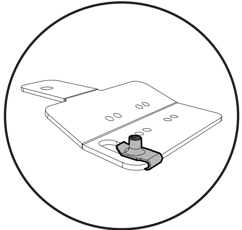
Install the ClipNut from the OEM plastic fender, onto the location shown. The OEM Flange bolt will also be needed.
