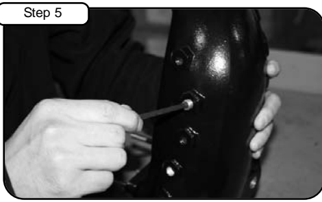
Step 5 Apply threadlocker to 1/8" NPT plugs. Install to aFe manifold using 3/16" allen key.
