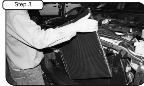
Pull up condenser only on the driver side.
