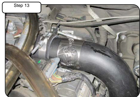
The charge air temperature may reach 400°F or higher at full load. Ensure wiring are routed away from intercooler tube. Your installation is now complete. Thank you for choosing aFepower!
