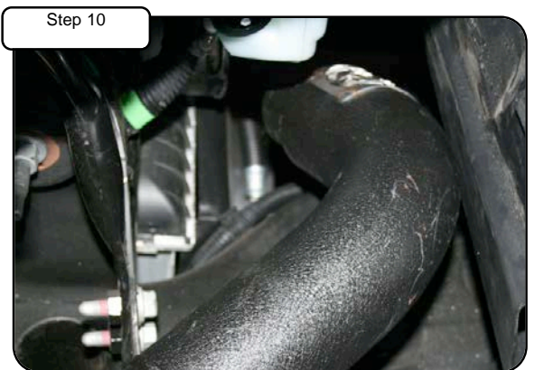
Install the new aFepower intercooler tube through the fender well. A second pair of hands guiding intercooler tube from above is highly recommended.
