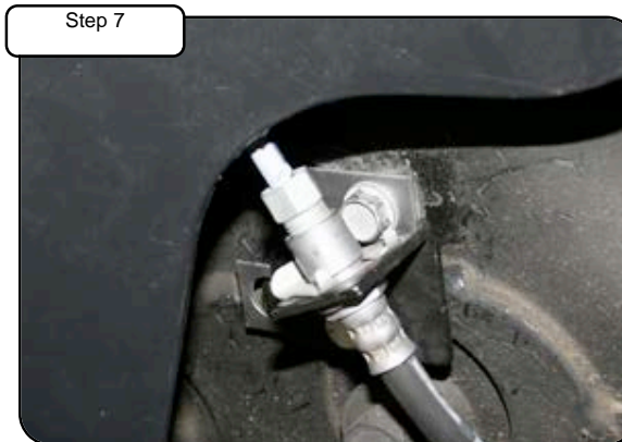
Install brake line bracket to the bracket adapter with M8 hex head screw and lock washer supplied.
