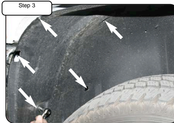
Remove the fasteners that attach the driver's side fender well forward portion. Pull back fender well and secure with steel wire or twine to access intercooler coupler.
