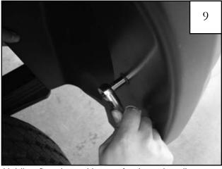
Holding flare in position on fender, reinstall screws removed in Step 8. Do not tighten. (An awl may be used to align the threaded clip with holes in flare and fender lip) Note: Make sure screws engage in splash shield.
