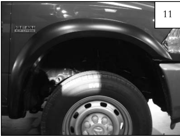
Completed front flare installation.
