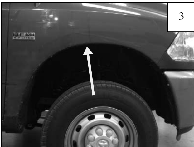
Install 1"x1.5" Black Tab and #10 U-Clip at this location. See steps 4, 5, 6, & 7.
