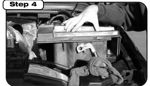
Remove battery terminals then remove battery lid. Wrap and isolate terminal or disconnect both batteries.
