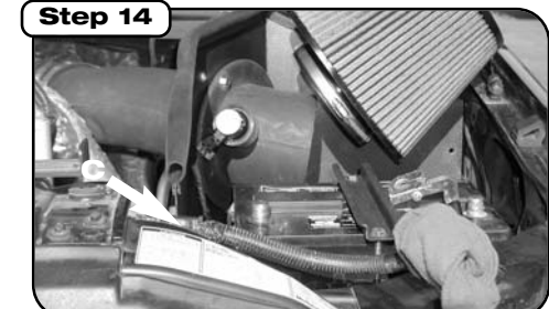
Install filter to intake tube and tighten clamp.
