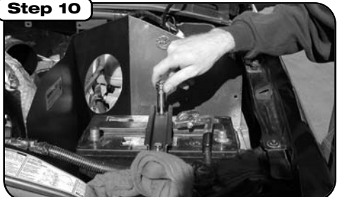
Place battery into intake housing using supplied clamp and two 8" long hex head bolts and locking washers. (DO NOT OVER TIGHTEN).
