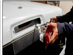
Remove factory 3<sup>rd</sup> brake light from vehicle.
