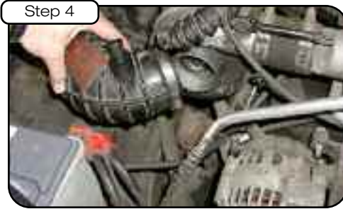
Remove factory rubber elbow at turbo.
