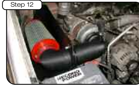
Complete aFe kit installed. Check and retighten all connections after first few hours of operation. NOTE: Place enclosed CARB EO sticker on or near the device on a smooth/clean surface. EO Identification label is required to pass the smog test inspection.
