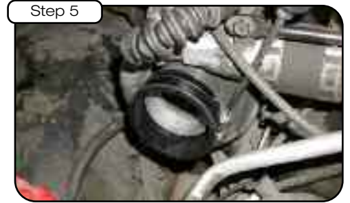
Place provided coupler onto turbo and secure the turbo end by tightening provided clamp.
