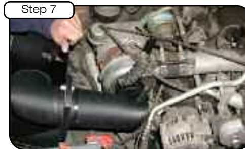
Before placing the heat shield into the engine compartment, slide the remaining clamp over the turbo coupler. Insert turbo end of the plastic tube into the coupler and rotate the assembly to seat the heat shield.
