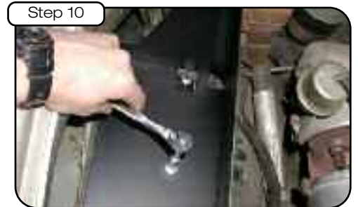
Using remaining M8 hardware and the existing holes in the fenderwell, secure the heat shield to the fender well. Tighten the hardware.
