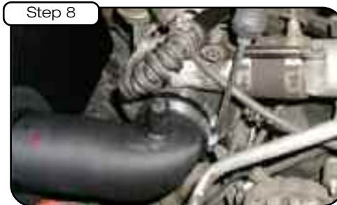
Tighten the remaining clamp securing the tube to the turbo coupler.
