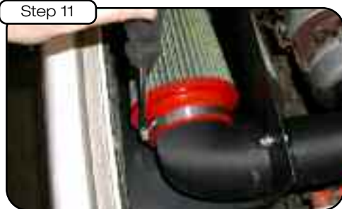
Install provided aFe filter onto the plastic tube and tighten.
