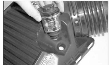
13. Remove the filter restriction gauge and grommet from the stock airbox as shown. **NOTE:** Use caution when removing gauge.
