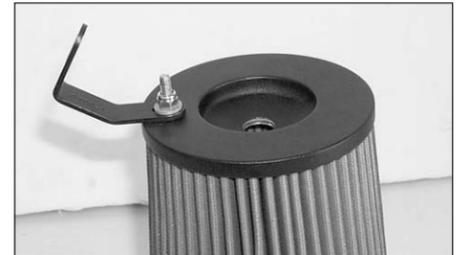
12. Install filter bracket provided onto the stud on the top plate of the Filtercharger element as shown. **NOTE:** Do not tighten completely.
