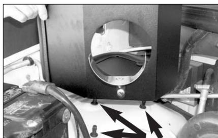
10. Install heat shield onto the locating studs as shown above.
