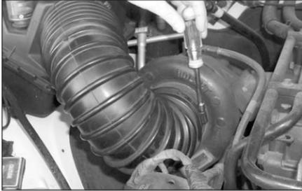
2. Loosen the hose clamp on the stock intake tube at the turbo.
