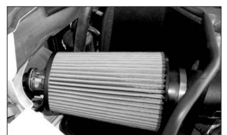
16. Install the Filtercharger element onto the intake tube. **NOTE:** Do not tighten completely.
