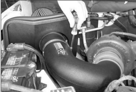
19. Attach saddle bracket to the intake tube with hose clamp provided. Adjust the bracket to achieve appropriate clearance for intake tube and tighten hardware.
