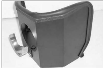
8. Attach the saddle bracket to heat shield using the hardware provided. **NOTE:** Do not tighten completely.
