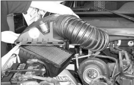
3. Release the 4 clips that retain the airbox top to the airbox base. Detach the intake tube from the flange on the turbo and remove the upper air intake assembly.
