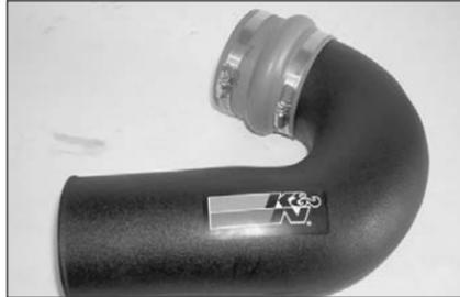
9. Attach the hump hose onto the K&N intake tube as shown.
