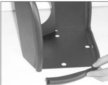
5. Install the edge trim on heat shield as shown. **NOTE:** Trim as needed.
