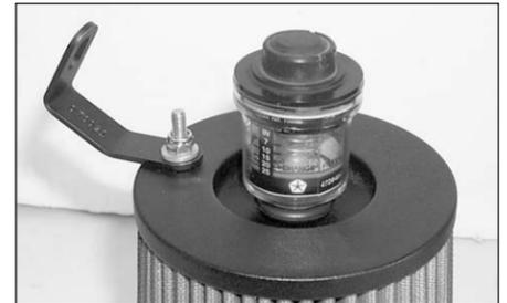
14. Install the grommet and restriction gauge into the hole in the top plate of the Filtercharger element.
