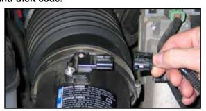
2. Depress the locking tab and then disconnect the Mass air sensor electrical connection.
