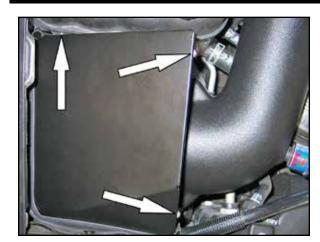
24. Install the filter cover onto the heat shield and secure with the provided hardware.
