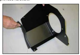
17. Install one of the 11" edge trims onto the heat shield as shown.
