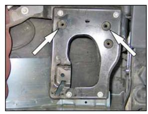
6. Remove the two air box mounting grommets shown from the air box mounting plate.
