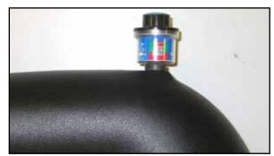
14. Install the filter minder and grommet into the  $K\&N^{\otimes}$  Intake Tube as shown.
