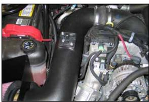
21. Install the K&N® Intake Tube into the silicone hose at the turbo inlet and into the heat shield, then secure the K&N® Intake Tube with the provided hose clamp and hardware as shown.
