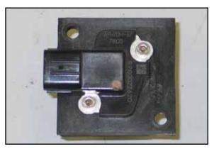
10. Install the mass air sensor into the adapter and secure with the provided hardware.
