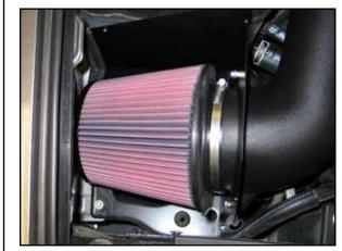
22. Install the K&N $^{\circ}$  Air Filter onto the intake tube and secure with the provided hose clamp.
