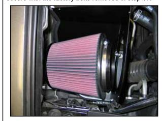
20. Set the K&N<sup>®</sup> Air Filter into the heat shield as shown.
