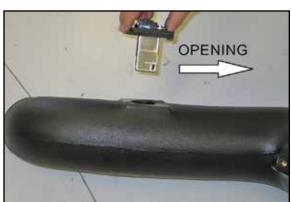
11. Install the mass air sensor assembly into the  $K\&N^{\tiny{\scriptsize{0}}}$  Intake Tube.
