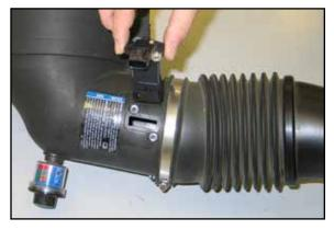
9. Remove the two screws that secure the mass air sensor onto the stock intake tube and then remove the mass air sensor as shown.
