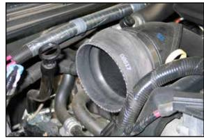
5. Install the provided silicone hose (08617) onto the turbo inlet tube and secure with the provided hose clamp.
