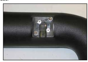
12. Secure the mass air sensor assembly to the K&N® Intake Tube with the provided hardware.
