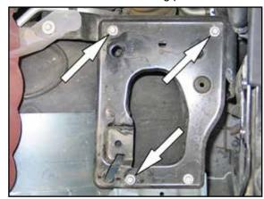
7. Remove the three air box mounting plate bolts shown.
