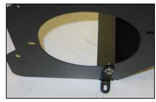
15. Install the "L" bracket (07805) onto the heat shield as shown with the provided hardware.
