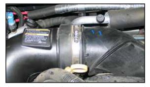
3. Loosen the hose clamp which secures the stock intake tube to the turbo inlet tube.
