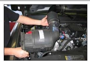
4. Disconnect the stock intake tube from the turbo inlet tube and then lift the complete stock intake assembly from the vehicle as shown.
