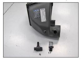
16. Remove the MAF sensors from the factory air box housing.
