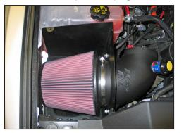
15. Install the K&N<sup>®</sup> intake tube into the heat shield and secure with the provided hardware. Then install the K&N<sup>®</sup> air filter onto the intake tube and secure with the provided hose clamp.
