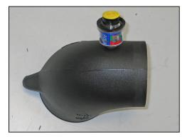
14. On vehicles that are equipped with a filter minder, install the provided grommet and the factory filter minder into the K&N<sup>®</sup> intake tube as shown. On vehicles not equipped with a filter minder, Install the provided plug.
