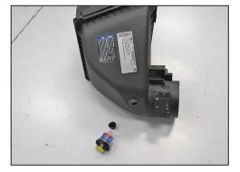
13. Remove the filter minder and grommet from the factory air box.
