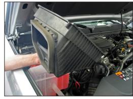
6. Lift up the lower air box to dislodge it from the mounting grommets and then remove the lower air box from the vehicle.
