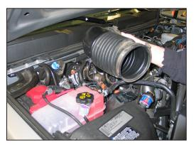
4. Remove the factory intake tube from the vehicle.
