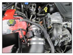
19. Install the mass air sensor assembly onto the  $K\&N^{\ensuremath{\circledast}}$  intake tube as shown and secure with the provided hose clamp.
