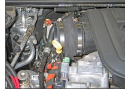
20. Install the provided hump hose (08617) onto the turbo inlet as shown and secure using the provided hose clamp.
