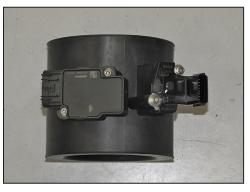
17. Install the mass air sensor into the K&N mass air sensor housing and secure with the provided hardware.
