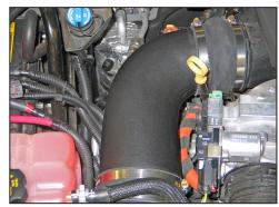
21. Install the K&N<sup>®</sup> intake tube into the silicone hose at the turbo inlet and then into the silicone hose at the mass air sensor. Adjust the tubes and mass air sensor housing for best fit and then secure with the provided hose clamps.
