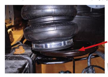
Slide the roll plate between the lower bracket and air spring while aligning the holes in all three.
