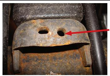
It will be necessary to tap the round hole in the forward driver's side spring perch. If there is no emergency brake cable bracket and mounting bolt as specified in Fig. 7 on the passenger's side, repeat and tap the round hole as instructed.
