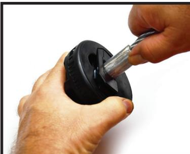
4. Secure the insert completely within the cavity.
