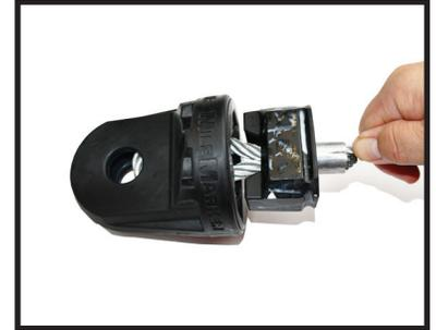
3. Apply two drops of lubricant to insert and spread evenly. Slip rope loop and insert into shackle mount cavity.
