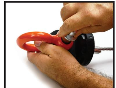
6. Thread shackle pin through rope loop, shackle eyelet, and shackle mount hole. Secure shackle as per normal operation.
