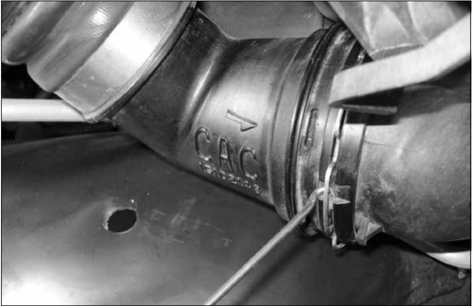
Figure 19 Passenger side boost tube
