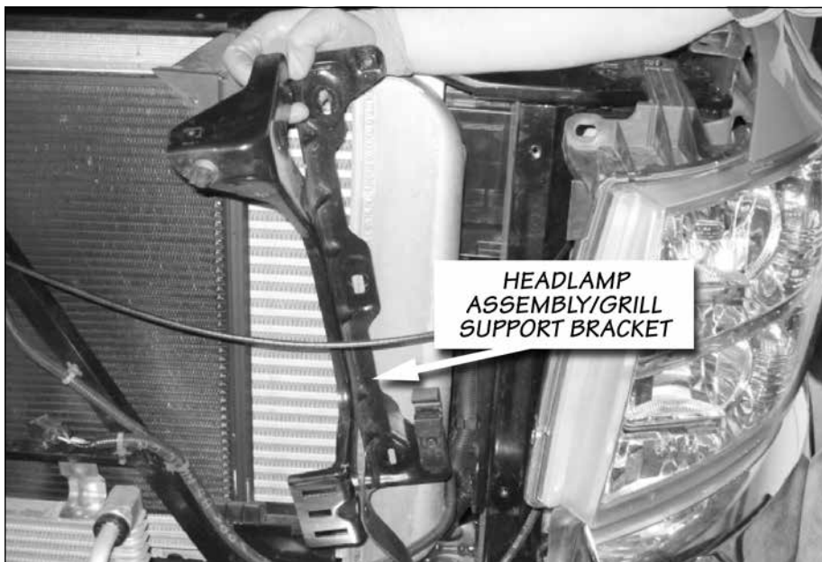
Figure 10 Headlamp Assembly/Grill support bracket
