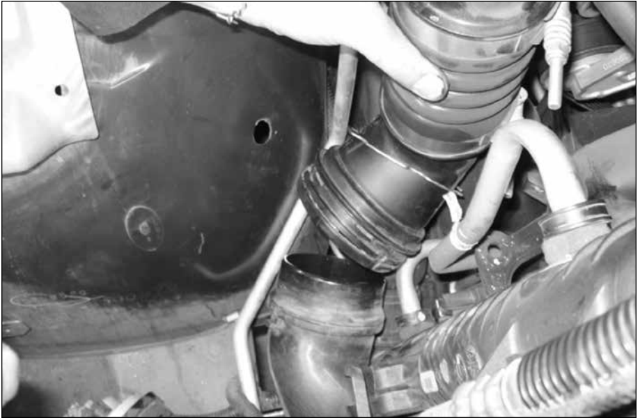
Figure 19 Passenger side boost tube
