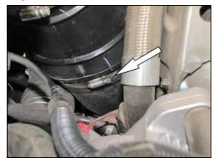
3. Loosen the hose clamp securing the intake resonator to turbo inlet hose.
