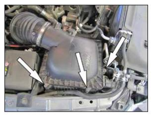
4. Remove the three screws securing air box lid.
