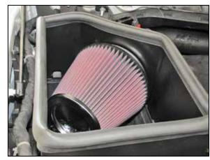
16. Install the K&N<sup>®</sup> air filter onto the filter adapter and secure with the provided hose clamp. NOTE: Drycharger® air filter wrap; part # RF-1042DK is available to purchase separately. To learn more about Drycharger® filter wraps or look up color availability please visit http://www.knfilters.com®.
