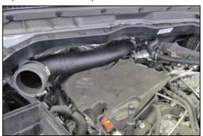
8. Install the K&N® intake tube into the factory turbo inlet hose and secure with the factory hose clamp.
