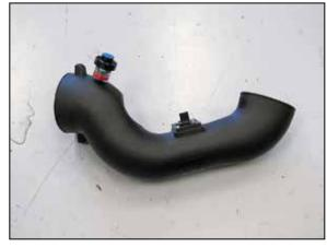
18. Install the filter minder using the provided grommet into the  $K\&N^{\circledast}$  intake tube.
