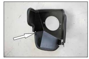
8. Using the provided hardware install one of the mounting studs onto the heat shield as shown.
