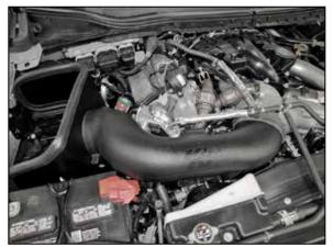
19. Install the intake tube into the heat shield and then into the coupling hose at the turbo inlet, adjust the tube for best fit and then install the provided bolts through the heat shield to secure the tube to the heat shield. Then secure the tube to the coupling hose with the provided hose clamp.
