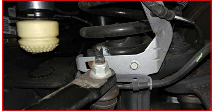
Install the ReadyLIFT brake line bracket to the factory brake line using **5/16" x 3/4" bolts, washers, and nuts**. Install the bolt with the head between the bracket and the frame. Torque to **10 ft-lbs**. Gently pull the metal brake line down while lining up the ReadyLIFT bracket to the original holes in the frame. Install using **factory hardware**. Torque to **5 ft-lbs**.
