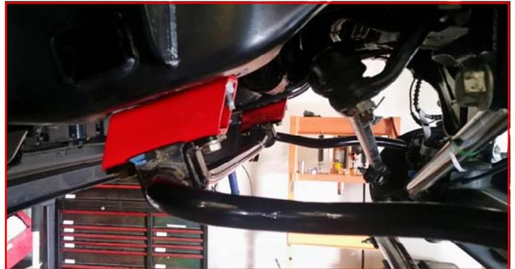
Install the ReadyLIFT shock extensions to the axle using factory hardware. Install the shock to the ReadyLIFT shock extensions using the **M14 x 70mm bolt, washers and nuts**. Torque to **45 ft-lbs**.
