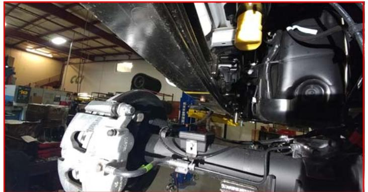
Locate the driver side lift block (Has a D cut into it under the bump stop tang). Raise the axle and the block up to the spring while aligning the center pin. **(If tapered, make sure small end points to the front of the vehicle.)** Install the **provided u-bolts, and nuts**. Snug the u-bolt nuts but do not fully tighten at this time. Repeat steps for passenger side.
