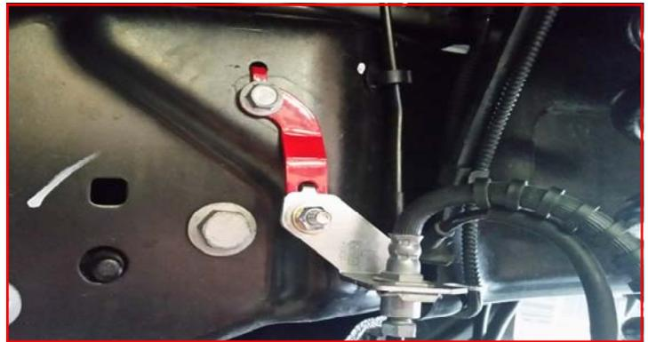
Remove the factory bump stop by pulling it out of its mount. Remove the mount from the frame.
