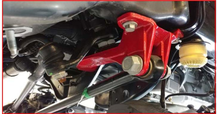
Lower the axle enough to remove the front springs. Install the ReadyLIFT urethane isolator, spring spacer, and then factory rubber isolator onto the spring. Raise the axle enough to hold the spring assembly in place.
