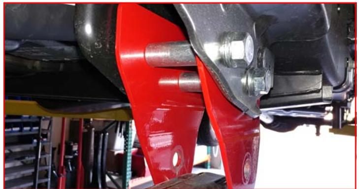
Rotate the axle until you can line up the radius arms into the ReadyLIFT drop brackets. Install using **factory hardware**. Do not tighten at this time.
