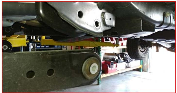
Install the ReadyLIFT radius arm drop brackets into the frame using **M18 x 130mm bolts, washers, crush sleeve, and nuts**. Do not tighten at this time.
