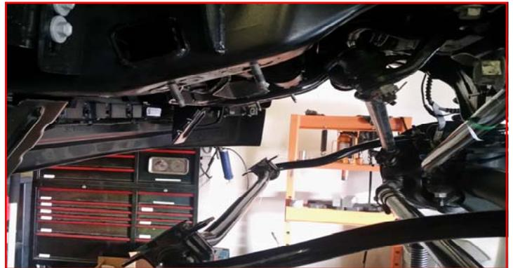
Remove the track bar from the factory bracket.
