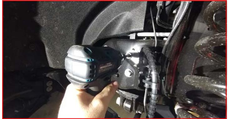
Remove the lower shock from the axle mount.
