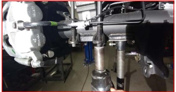
Lower the axle just enough to remove the factory block and install the ReadyLIFT block, making sure not to over extend brake and ABS lines. Adjust as necessary.
