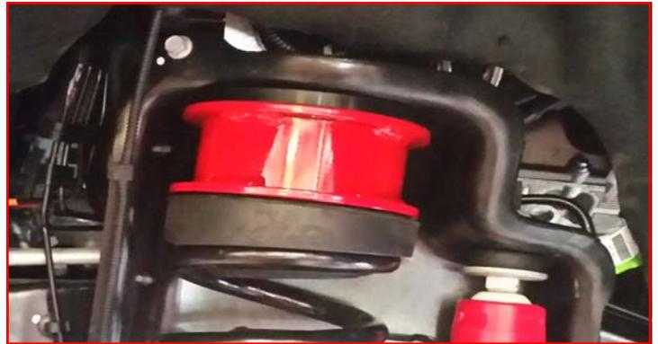
Install the ReadyLIFT sway bar drops to the frame using factory hardware. Torque to **35 ft-lbs**. Install the sway bar to the ReadyLIFT sway bar drops using the **7/16" x 1 1/2" bolts, washers and nuts**. Torque to **35 ft-lbs**.
