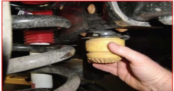
Install the ReadyLIFT bump stop spacer and factory bump stop mount to the frame using **M8 x 70 mm bolt and washer**. Torque to **5 ft-lbs**. Install the bump stop to the factory mount by pressing it back into place.
