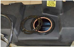
(Fig. 1) Remove sending unit from original equipment tank using mallet or hammer and large screwdriver.
