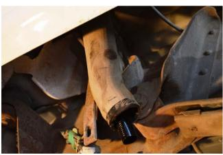
(Fig. 10) On vehicles with LB7 engines only, an interior fill hose is located inside the main fill hose. The tank vents through the space provided between the two hoses. Ten (10) inches needs to be cut off of the <u>interior</u> hose on end that goes to the tank as shown.
