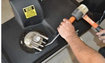
(Fig. 3) Make sure the sending unit tab lines up with the "tab location" mark.
