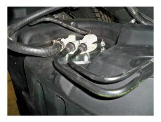
(Fig. 12) Lift tank high enough to reconnect electrical cable and vent hose to sending unit.
