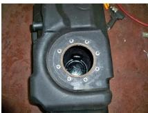
(Fig. 3) Leave the "O" ring gasket, studs and retainers assembled as they are (shown before sending unit, top flange, and 3/8" nylon Locking nuts are installed).
