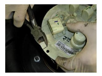
(Fig. 5) If sending unit connections interfere with the mounting studs, trim  $\frac{1}{2}$ " off the side of the tab nearest the electrical connector.
