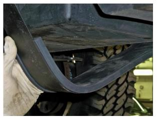
(Fig.13) Extruded bushings installed on straps
