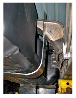
(Fig. 15) Hanger Bracket installed on frame
