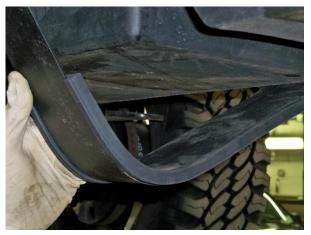
(Fig.13) Extruded bushings installed on straps.
