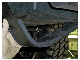
(Fig.12) Extruded bushings installed on straps.
