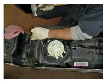
(Fig. 2) Loosen hold-down ring on OEM tank by tapping counter-clockwise, remove and lift out sending unit.
