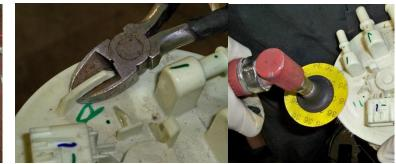
(Fig. 4) If sending unit is equipped with curved ribs on the top, either shave approximately 1/16" off the outside surface of both, or remove the rib closest to the electrical plug using dikes and a hand grinder-sander as shown above so top flange will fit correctly. **Be sure surface is perfectly smooth and even to prevent breakage when top flange is tightened.**
