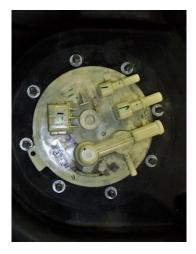
(Fig. 6) Be sure the sending unit is "clocked" nearly the same as in the OEM tank. If the tab was trimmed as in Fig. 5, place the sending unit and rotate it slightly more clockwise until it clears the studs as shown.
