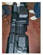
(Fig. 8) Attach the fuel lines to the sending unit and lay them in the retaining groove provided on the top of the replacement tank.
