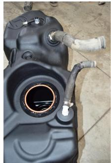
(Fig. 5) Using a hammer and punch, or screwdriver tighten the locking top ring clockwise. The short feed line is shown installed in photo.
