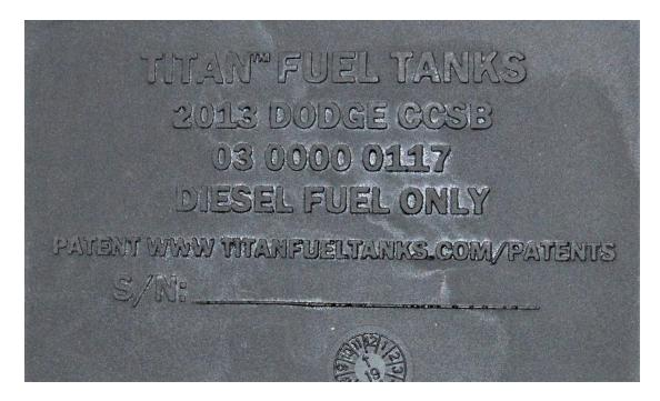
**Note:** The tank body has the above identification on its bottom. Please check to be sure the tank is properly identified as the one to fit your vehicle. Notice the serial number space. You will need the serial number to register for warranty coverage.
