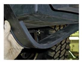
(Fig. 5) Install rubber bushings (pn 99 0000 0103) on both straps and the front Support with the channel side toward the strap.
