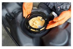
(Fig. 3) Place the sending unit into the TITAN tank and place the Torque Ring hold-down ring on top, threading it onto the lugs. Tighten the ring by turning it clockwise as far as it will go
