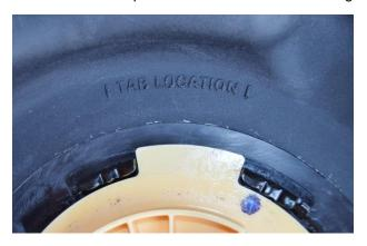
(Fig. 4) Be sure the tab on the sending unit lines up with the "TAB LOCATION" marks on the tank body as shown above.
