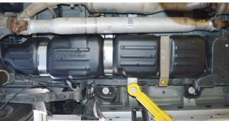
(Fig. 12) You might want to straighten the tank straps a little to aid in installation.
