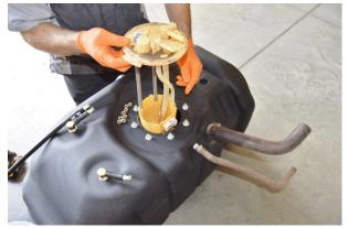
(Fig. 7) Place the sending unit in the TITAN Tank.
