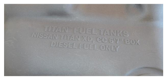
**Note:** The tank body has the above identification on its top. Please check to be sure the tank is properly identified as the one to fit your vehicle.
