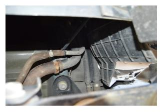
(Fig. 1) Loosen and disconnect fill hose and vent line from vehicle's fill spout.
