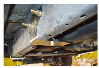
(Fig. 15) Front Support Bracket Installed.
