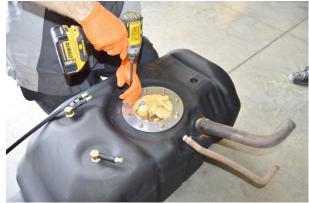
(Fig. 8) After placing the sending unit into the TITAN tank, install the top flange, and tighten the nylon lock nuts to 20 lb. ft. using a "star" pattern using a torque wrench.
