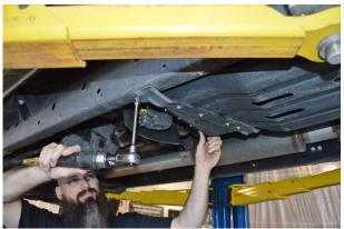
(Fig. 2) Remove factory shield.
