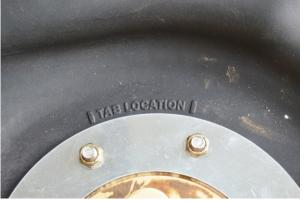
(Fig. 6) Line the tab on the sending unit up with the "tab location" mark on the TITAN tank.
