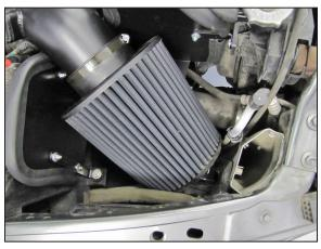
26. Install the K&N $^{\mbox{\tiny 0}}$  air filter and secure with the provided hose clamp.
