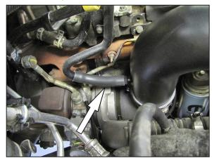
25. Install the provided crank case vent hose onto the fitting installed into the  $K\&N^{\textcircled{0}}$  intake tube and
