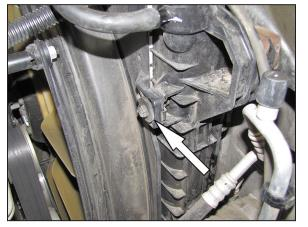
16. Remove the fan shroud bolt shown.
