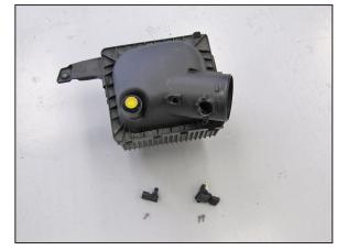
18. Remove the mass air sensor and inlet air temperature sensor from the factory air box as shown.
