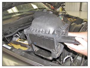
6. Remove the complete air box from the vehicle as shown.
