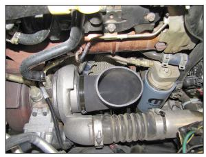
8. Install the K&N<sup>®</sup> elbow hose onto the turbo inlet and secure with the provided hose clamp.
