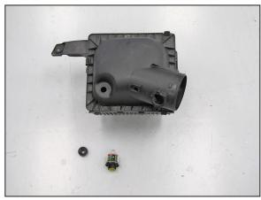
19. On vehicles equipped with a filter minder, remove the filter minder and factory grommet from the air box as shown.
