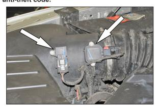
2. Disconnect the Mass air sensor and temperature sensor electrical connections, and then unhook the wiring harness from the air box.
