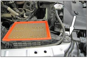
5. Remove the bolt which secures the lower air box to the core support.
