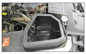
11. Install the air box so the mounting studs insert into the air box mounting grommets and then secure the air box to the mounting bracket installed in step #8. Tighten the mounting bracket bolts.
