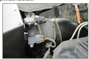
19. Reconnect the mass air sensor and temperature sensor electrical connection.
