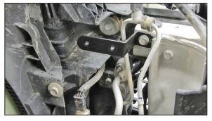
8. Install the air box mounting bracket (083145) onto the core support using the bolt removed in the previous step.
