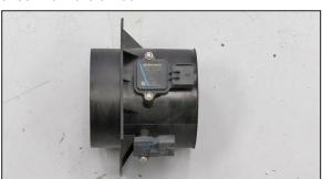
13. Install the mass air sensor and map sensor into the K&N® mass air sensor housing using a twisting motion to aid installation and then secure with the
