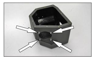
9. Install four of the provided 6mm studs into the  $K\&N^{\circledast}$  air box as shown.
