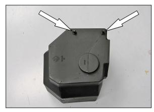
10. Install the two provided air box mounts to the bottom of the air box and secure with the provided hardware.
