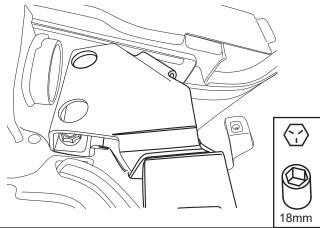
Reinstall support bar (removed in step 2) and slide support bracket (6) over stud. Use supplied hardware (7) to bolt strap to assembly.
