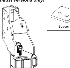
Remove support bar with a 21mm deep socket and a 13mm socket or wrench.
