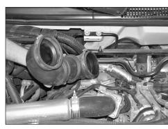
7. Loosen the hose clamp that secures the intake tube assembly to the turbo inlet tube. Then remove the complete inlet tube assembly from the vehicle as shown.
