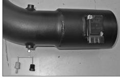
10. On vehicles equipped with a filter minder, install the 1/4" npt vacuum fitting into the K&N<sup>®</sup> intake tube. On vehicles not equipped with a filter minder, install the 1/4" npt plug into the K&N<sup>®</sup> intake tube.
