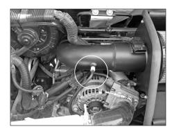
25. On vehicles equipped with a filter minder, connect the vacuum line to the  $\frac{1}{4}$ "npt fitting installed in the K&N intake tube as shown.
