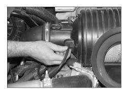
3. On vehicles equipped with a filter minder, disconnect the filter minder vacuum hose from the stock filter housing.
