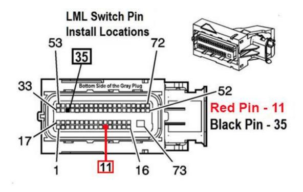
Note: Some Tuner could use different Pin locations, confirm to ensure proper pin locations and Installation
