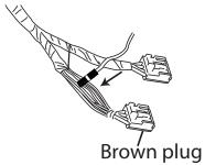
Reassemble door and replace plugs. Plugs must be replaced for Power Step to operate.
