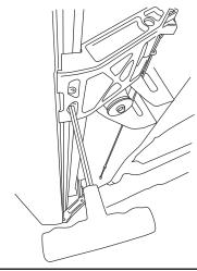
Using a 13mm socket Torque linkage bolts 4x (8) from step 3 to 16 ft-lbs. Next use a 10mm socket, torque linkage spacer bolt 2x (12) from step 5 to 8 ft-lbs.
