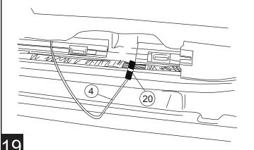
**REAR DOORS** - Carefully remove wire wrap and find LIGHT BLUE wire with BLACK STRIPE. On passenger side find GREEN wire with BLACK STRIPE. The wire is located rear of the "T" junction where wires cross under the front seat.
