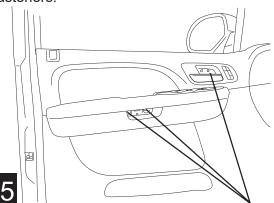
Remove door latch cable from door panel.
