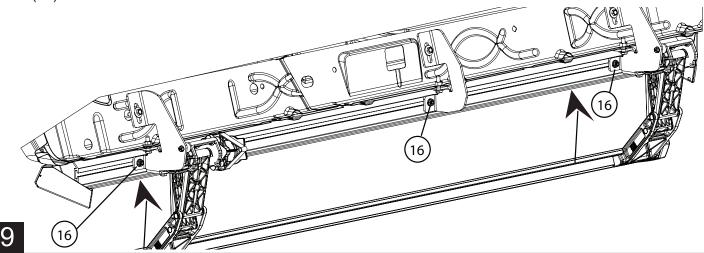
**A**: Using a 13mm socket tighten 3 bolts along pinch weld first. Torque to 16ft-lbs.
