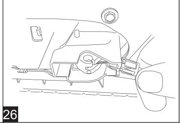
Pull back the door weather guard, unbolt speaker and unplug. Thread plastic tube through accordion.
