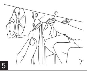
Install provided spacer (17) and M6 bolt (12) into upper mount as shown on both the Drive and Idler linkages. Do not tighten.
