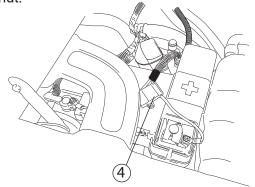
Attach ground lead to negative battery pole.
