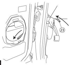
Feed longer wire of Step 13 through tube into door and pull out plastic tube on door side. Route wire along harness to switchplate.
