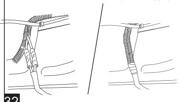
Attach motor to harness using a 4mm Hex Torque to 36 in-lbs. Connect harness to motor. Secure harness with tie wraps.
