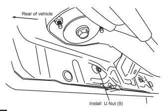
Set rail up into position. Starting with the rear bracket work towards the two front brackets. Attach Bolts 2x (8) and Nut 1x (9). Snug to body do not tighten!
