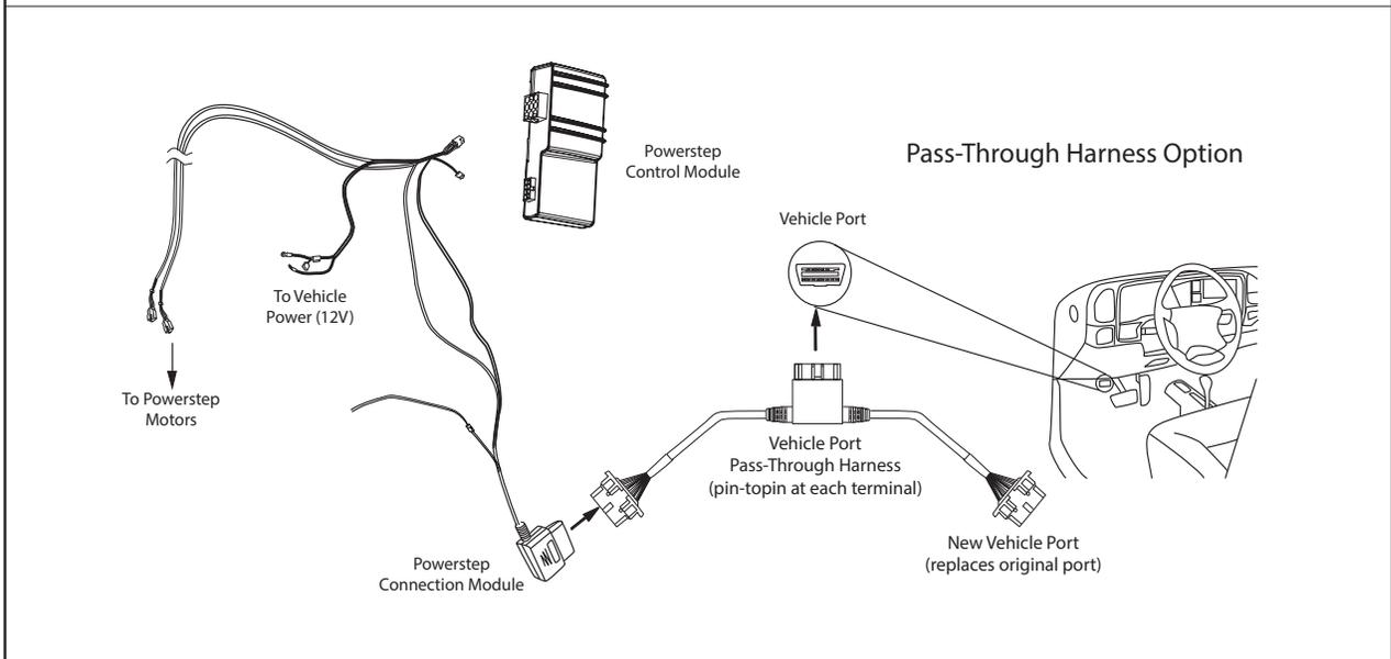
On driver side, run Wire Harness leg down and along underside of the vehicle floor and frame to front Drive Linkage. Connect harness to motor and secure harness with tie wraps. Route remainder of wire harness towards rear linkage assembly for LED lights. Repeat step on passenger side.
