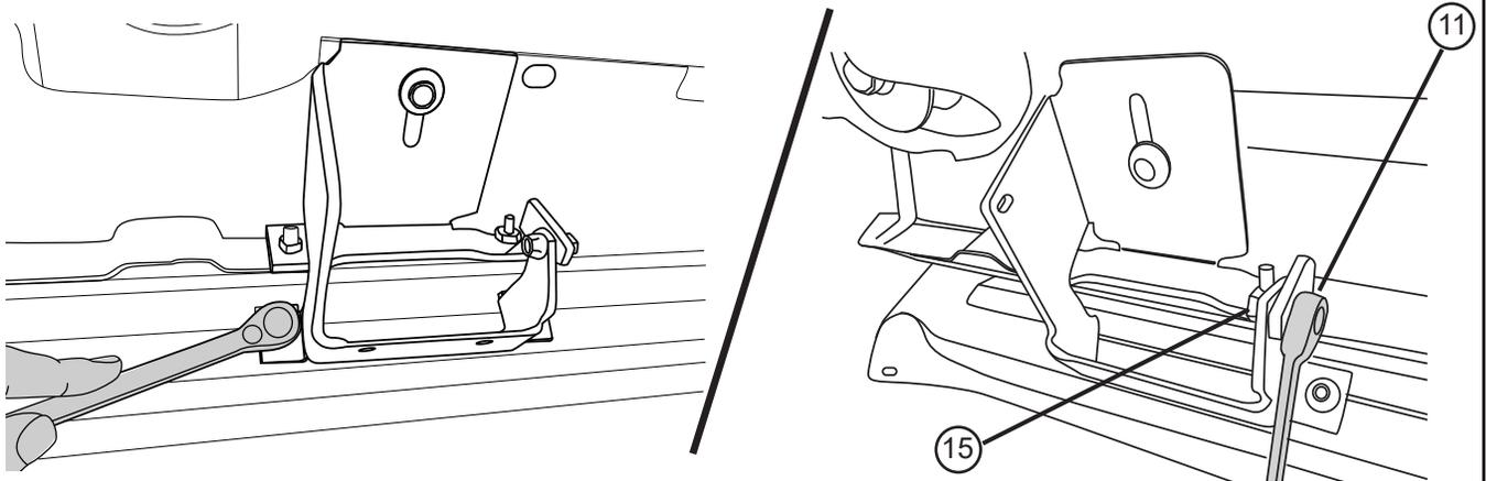
Attach rail support bracket (27) by inserting carriage bolt (15) into rail from the front of vehicle side, use flange nut (17) to attach it. Using supplied button head bolt (11), washer (19) and captive washer nut (18) to pinch weld. Torque bolts to 16ft-lbs.
