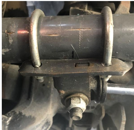
Figure 7. Installed Tie Rod Clamp and Steering Stabilizer
