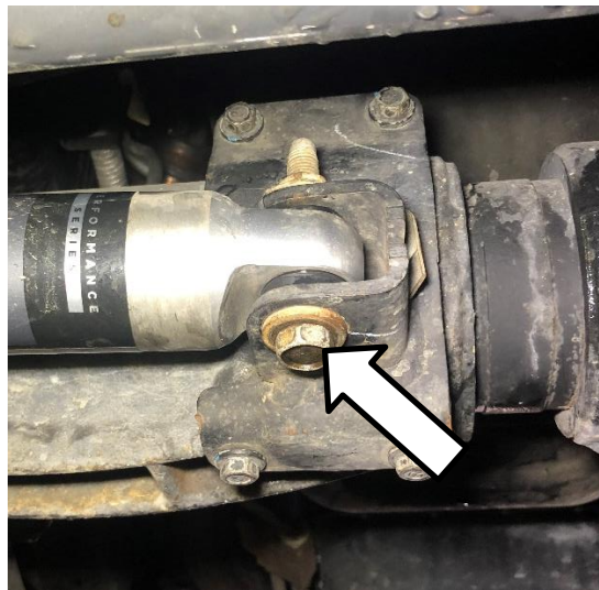
Figure 1. Stabilizer Bolt to be Removed
