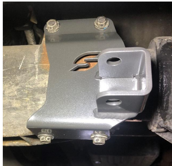
Figure 3. Loosely Installed Synergy MFG Stabilizer Relocation Bracket
