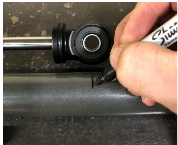
Figure 6. Mount Centerline Marking
