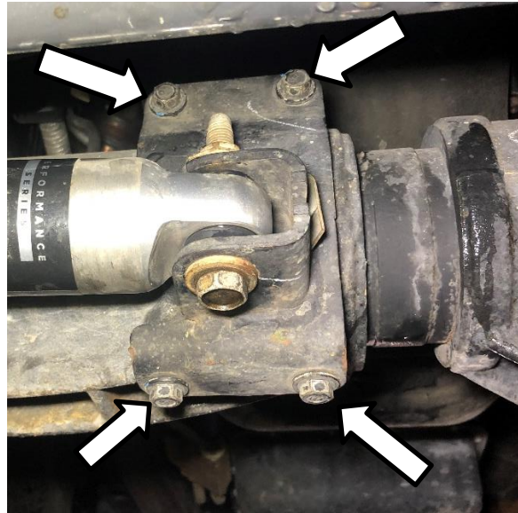
Figure 2. Bolts to Remove Factory Stabilizer Mount
