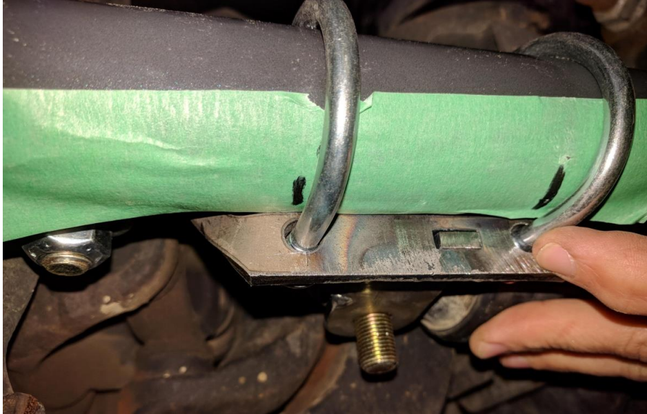
Figure 4. Clamp Centered on Tie Rod
