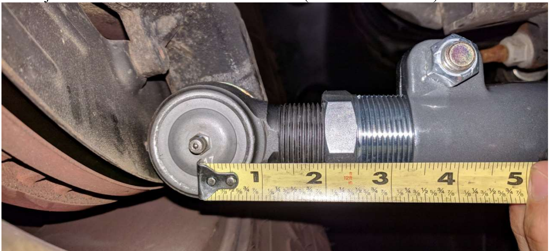
Figure 8. Double Adjuster Tie Rod End Max Extension
