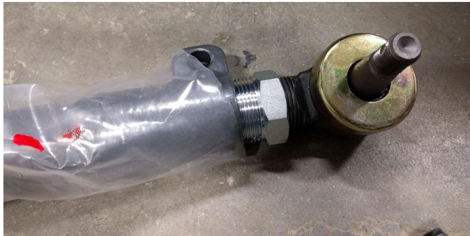
Figure 3. Double Adjuster Side of Tie Rod
