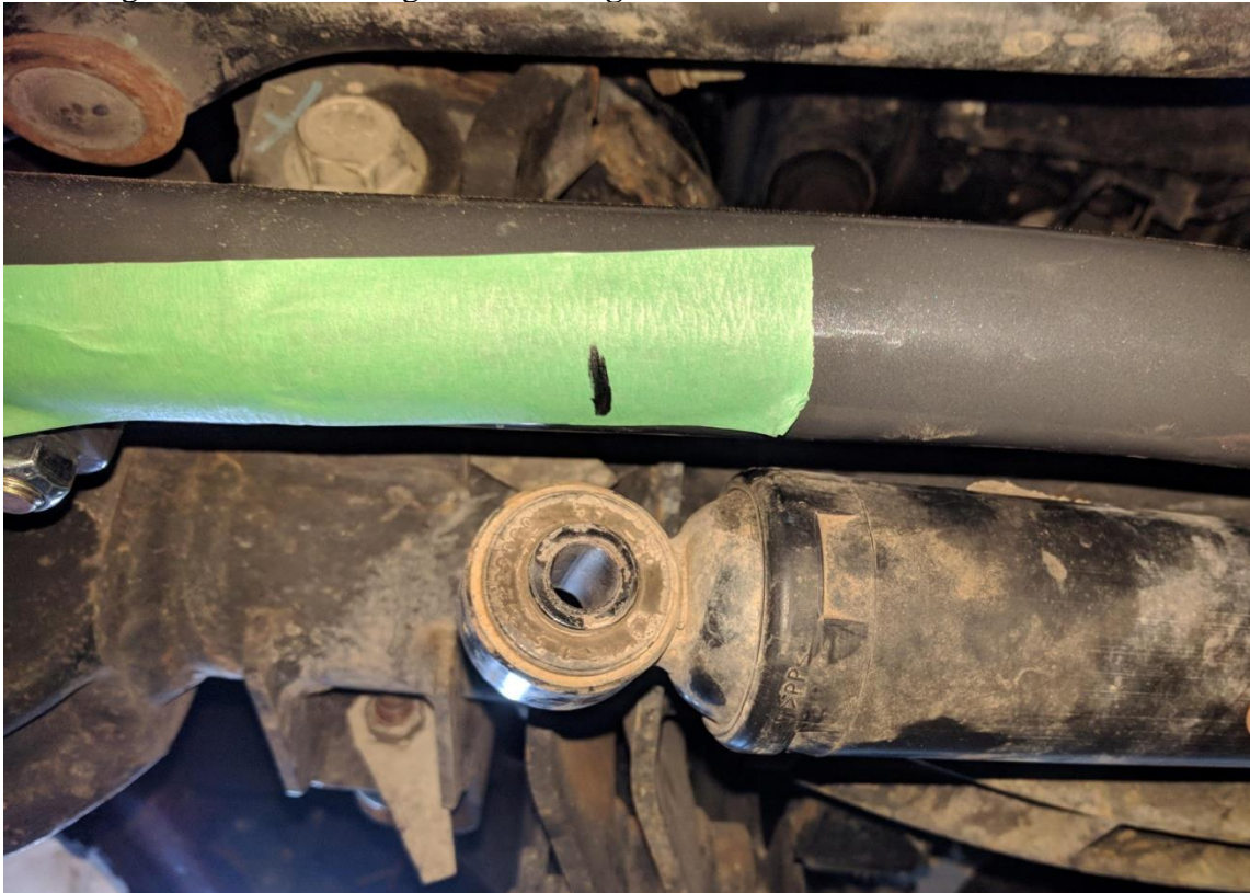
Figure 1. Steering Stabilizer Fully Collapsed, Steering Full Lock Driver
