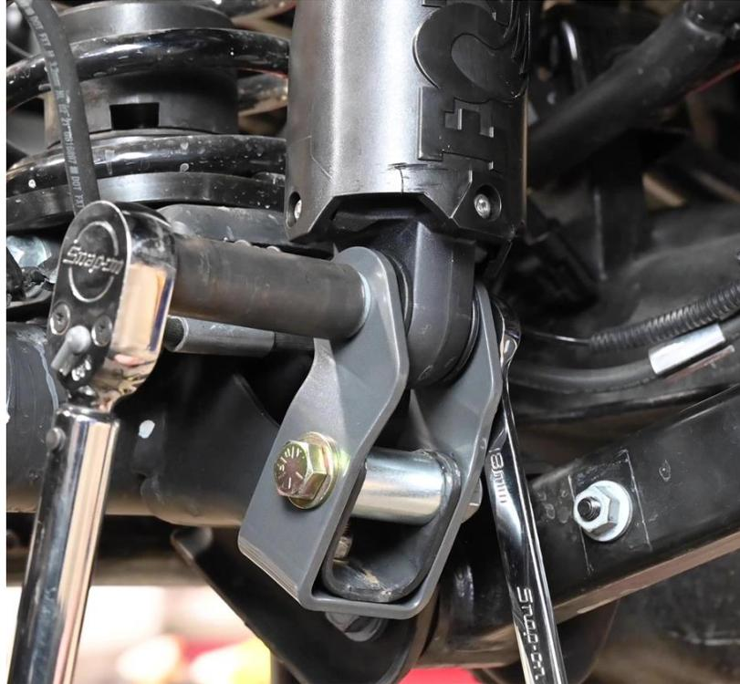
**Figure 3. Bolting Shock to Extension**
