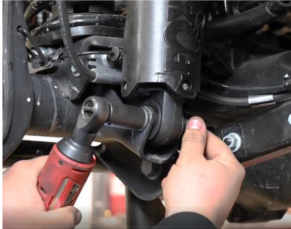
**Figure 1. Removing Lower Shock Bolt**
