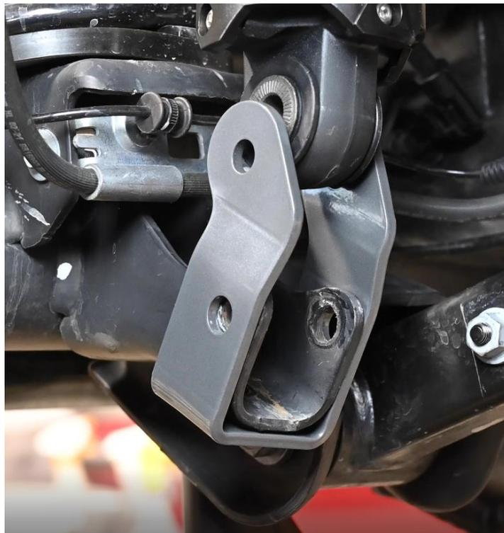
**Figure 2. Shock Extensions Installed**
