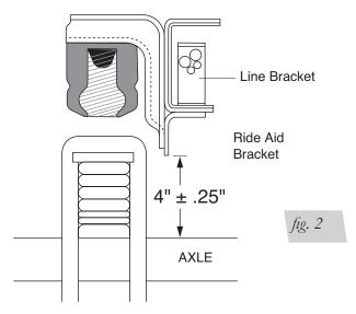
Normal Ride Height is the distance between the bottom edge of the wheel well to the center point of the hub with the vehicle in an "as delivered condition" (without a load, i.e. tool box, camper, etc.). Measurements should be taken before beginning the installation. The distance from the bottom edge of the wheel well to the center point of the hub should be recorded. This kit is designed to be installed and operated at normal ride height.
