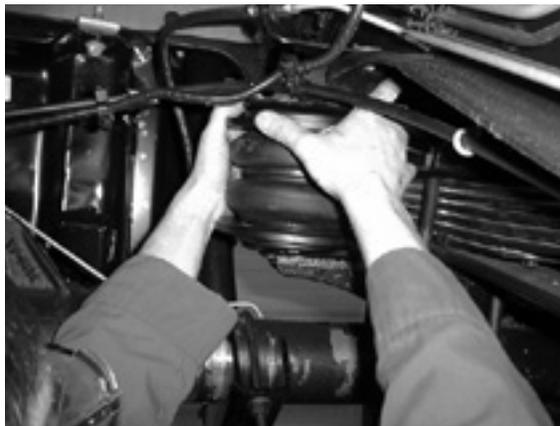
8. As in the previous step, move the bottom bracket inward and outward so as to align it with the bellows and the upper bracket (Fig. 14).
