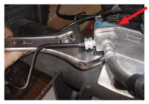
Bend bracket 1/8" (3mm) to gain clearance for the ABS line once the air spring assembly is installed.
