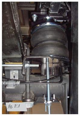
Driver's (left) side rear view of kit installed.
