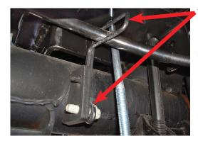
The wire emergency brake cable hanger may need to be moved forward slightly to clear the lower bracket.
