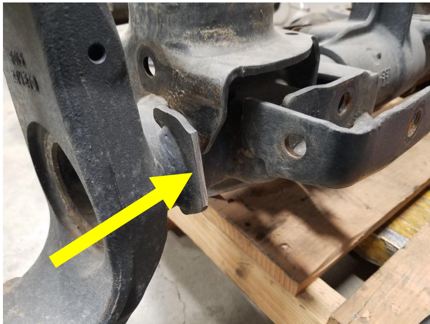
Figure 1. Removing Outer Passenger Side Sway Bar Tab
