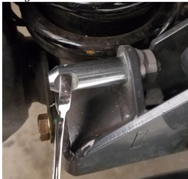
Figure 6. Passenger Side (Right) Disconnect Stud Installed with 8855-01 Front Track Bar Relocation Bracket
