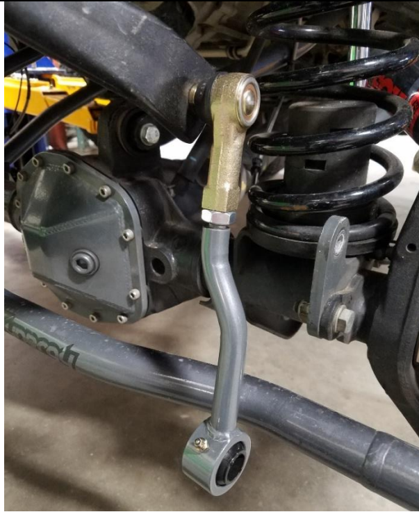
Figure 4. Correctly Installed Driver's Side (Left) Sway Bar End Link
