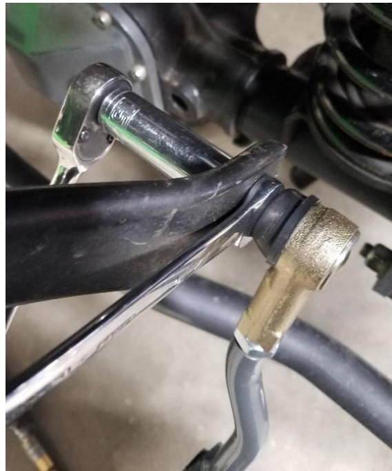
Figure 3. Installing the Driver's Side (Left) Sway Bar End Link
