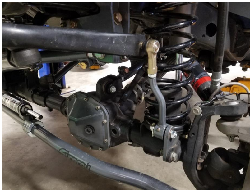
Figure 14. Correctly Installed and Connected Link (Driver's Side)
