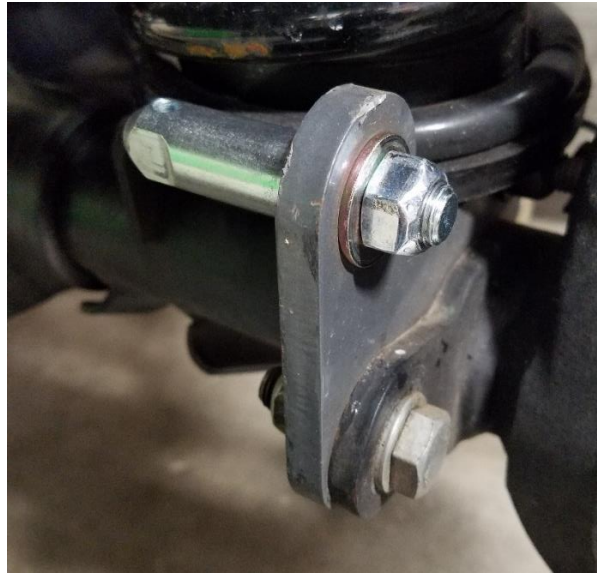
Figure 5. Disconnect Stud Installed in Relocation Bracket
