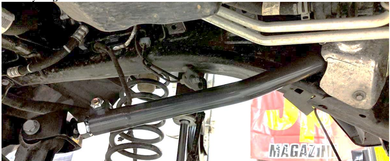
Figure 4. Synergy MFG Right-Side Control Arm Installed With Heat Shield
