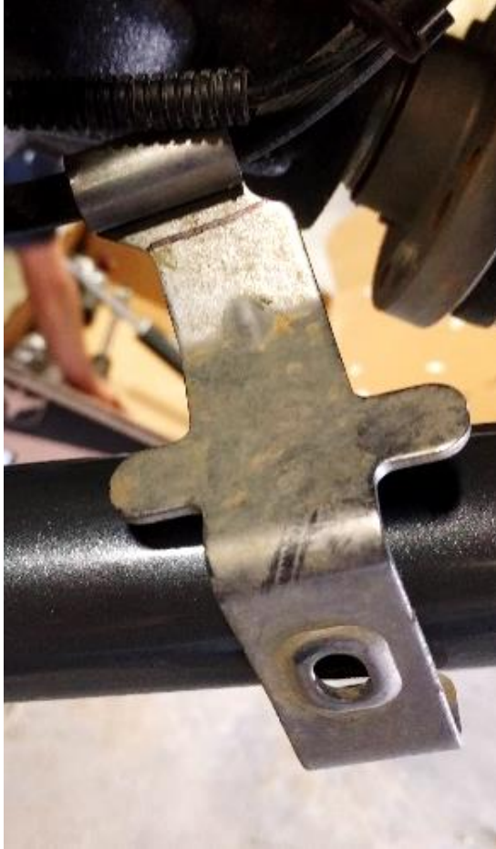
Figures 1 and 2. Marking and Trimming Factory Brake Line Bracket
