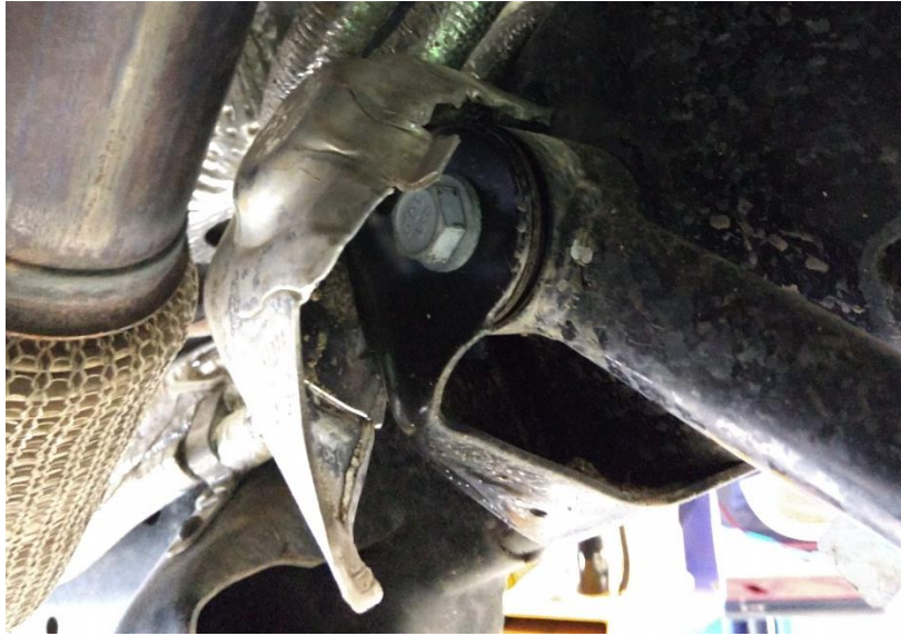
Figure 1. Front Upper Control Arm Heat Shield Bent Out
