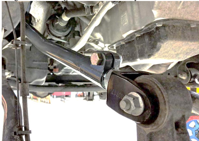
Figure 2. Correctly Installed Synergy MFG Right Front Upper Control Arm
