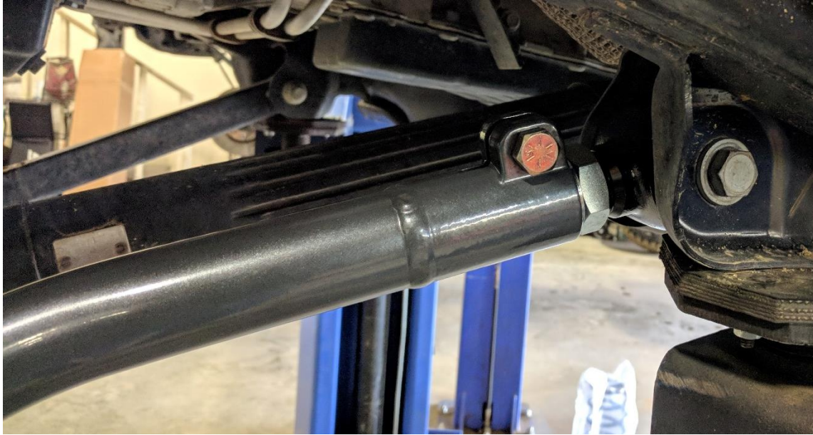
Figure 4. Control Arm Correctly Installed (Frame Side Shown)
