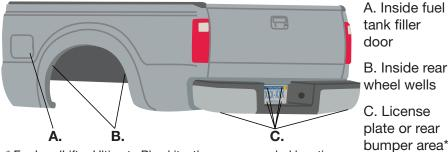
\* For LoadLifter Ultimate Plus kits, the recommended location for the Schrader valves is the rear bumper area or license plate.
