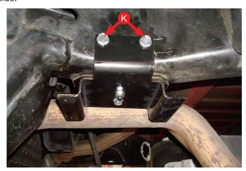
Driver's side bracket shown mounted in place and ready for the air spring assembly.
