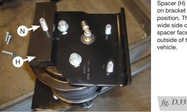
Spacer (H) set on bracket in position. The wide side of the spacer faces the outside of the vehicle.
