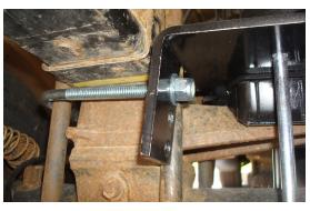
Evenly tighten only enough to draw the lower bracket to the Stock U-bolts at this time.
