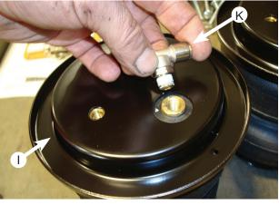
Set roll plate (I) over the air spring and install the fitting (K) as stated. Repeat for both air springs.
