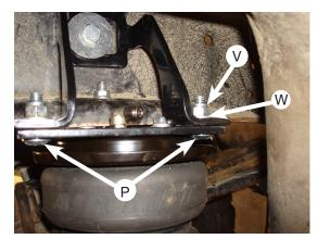
Cap the 3/8"-16 x 1.25" carriage bolts with 3/8" nylon lock nuts and torque to 15 lb.-ft. (20Nm) Repeat for both sides.
