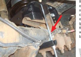
It may be necessary on some models to not tighten the axle clamp bar evenly on the right side (passenger's side) so that the clamp bar will clear the hard brake line.
