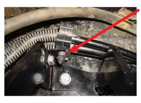
Insert the line holder previously removed into the L-bracket installed on the upper brace as shown.
