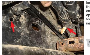
Image shows lines clear on the frame opening it up for the brace installation.
