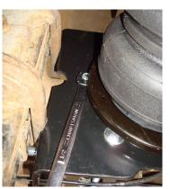
Tighten lower main plate/swivel cup mounting hardware once the lower bracket is in position and tight.
