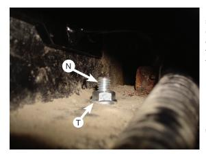
Install the 3/8"-16serrated flange lock nut (T) onto the  $3/8"-16 \times 2"$ carriage bolt (N) that goes through the flange on the frame and tighten.
