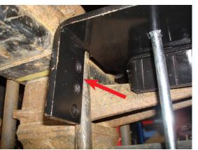
Rotate the lower bracket on the jounce bumper strike plate if necessary and push the bracket up against the U-bolts to put the lower bracket into position.
