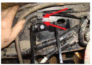
Brace being temporarily held in place by the M8 bolt and washer. L-bracket is shown in location already. Note: The side the line holder is on depends on the location of the factory retaining clip.
