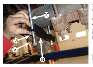
Set the axle clamp bar over the 3/8"-16 x 10" carriage bolts and cap with 3/8" flat washer and 3/8" nylon lock nut. Leave loose at this time.
