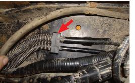
If equipped, this emissions/fuel line holder must be pulled away from the frame in order to install the upper frame brace (E).
