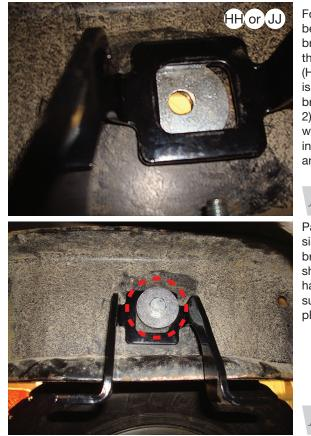
For the passenger's side, before inserting the upper brace hardware, make sure that the 1/2" thick washer (HH) or 3/4" washer (JJ) is installed in between the brace and frame (see Step 2). Note: The 1/2" thick washer (HH) is not a half inch thick. It has a 1/2" hole and is a thick washer.
