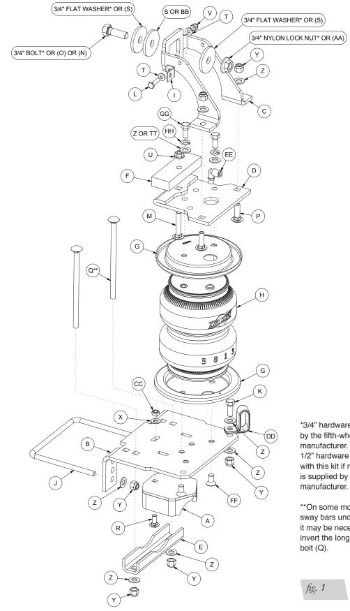
\*3/4" hardware is supplied by the fifth-wheel hitch manufacturer. Use the 1/2" hardware supplied with this kit if no hardware is supplied by the
