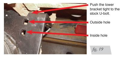
If installing this kit on a single-rear-wheel (SRW) vehicle, use the inside position square holes in the lower bracket to insert the long 3/8"-16 x 10" carriage bolts (Q) through (Fig. 19). If installing this kit on a dual-rear-wheel (DRW) vehicle, use the outside set of holes to insert the carriage bolts through.
