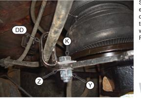
Secure the emergency brake cable away from the air spring with the modified P-clamp (DD).
