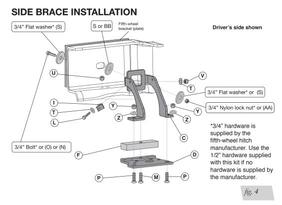
1. Set the upper brace (C) into the driver's and passenger's side frame (Fig. 4).
