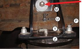
Torque both sides to 44 lb.-ft. (60Nm).
