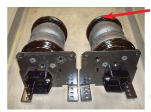
The fitting should be on the top or this side of the air spring assembly (opposite of flanges on lower bracket).
