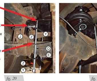
Depending on the truck model, the carriage bolt might go between the brake line and axle or outside the brake line.
