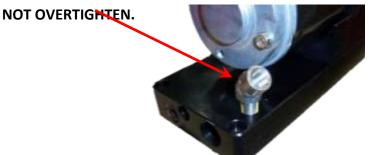
3. Install the pressure switch (5C-9-007) into the 45° elbow fitting (4A-5-02-02S) as shown below. **DO NOT OVERTIGHTEN.**
