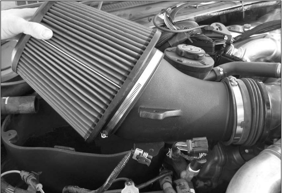
**(Figure 13)**. Tighten the Screws with a #3 Phillips screwdriver.
