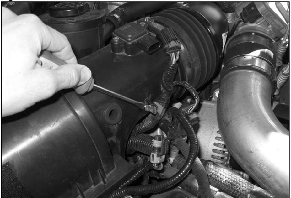
**9.** Push the air cleaner bellows away from the air filter housing while pulling up on the MAF side of the air filter. Lift and remove the air filter housing in the direction shown in **Figure 7**.
