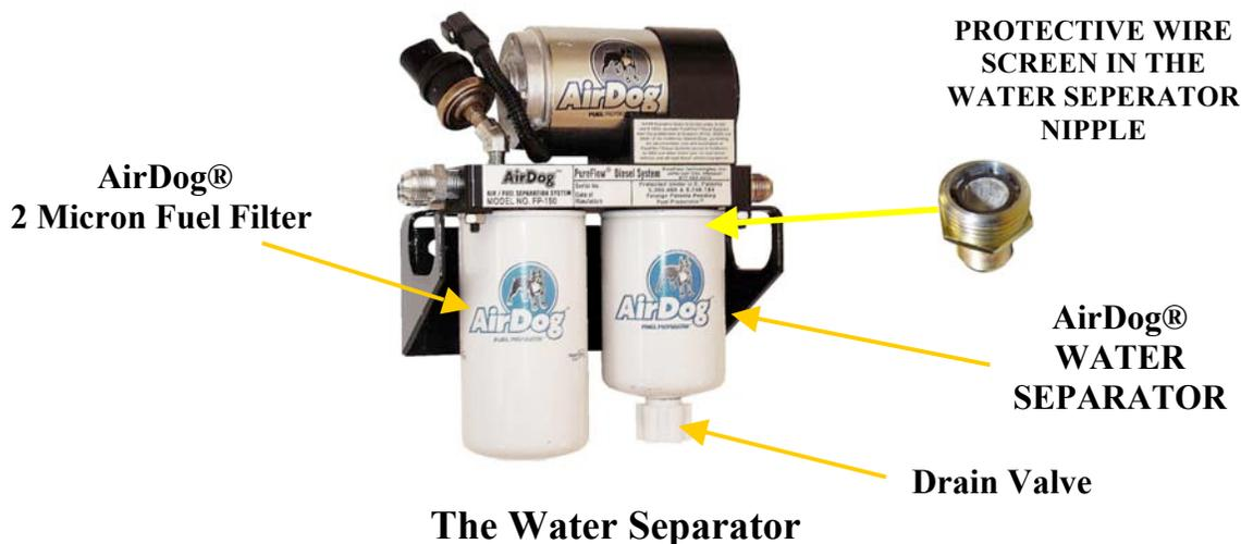
Replace the water separator every other time you change the Fuel Filter or if it becomes damaged or plugged. It is suggested to check/drain the water separator every three months or as needed should you experience excessive ‘water in fuel’ conditions. When installing the water separator, be sure to clean the under side of the AirDog® base. Follow the instructions printed on the pre-filter for proper tightening procedures.
