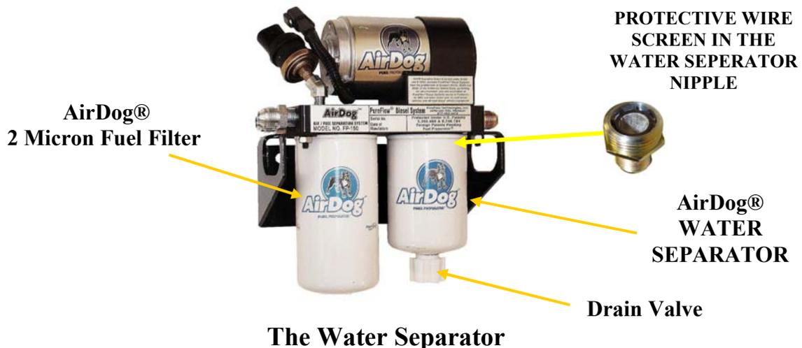
Replace the water separator every other time you change the Fuel Filter or if it becomes damaged or plugged. It is suggested to check/drain the water separator every three months or as needed should you experience excessive 'water in fuel' conditions. When installing the water separator, be sure to clean the under side of the AirDog® base. Follow the instructions printed on the water separator for proper tightening procedures.
