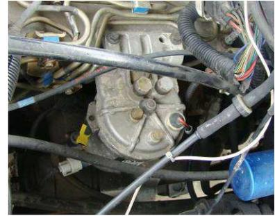
**NOTE:** Be sure to keep the ORIGINAL ENGINE RETURN LINE connected as it is from the factory! In many cases the return runs thru the flange of the filter canister.
