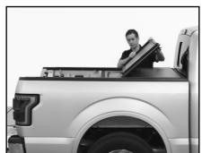
C. Always ensure all latches and hooks fully engage side rails. Close tailgate.
