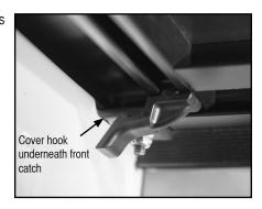
B. With cover hooks engaged underneath front catches, lower cover to engage latches in retainment brackets on each side.
