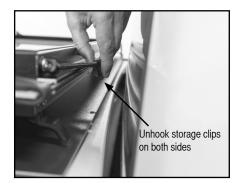
E. Unfold rear panel toward tailgate. Hooks on rear panel will automatically engage rear catches on each side. Latches will automatically engage each side rail at rear of box. Ensure all latches fully engage side rails when closing cover.
