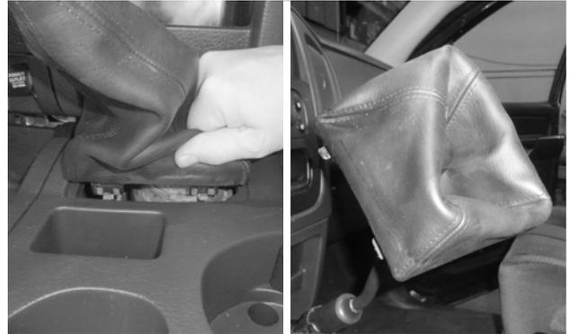
1. **Shift the transmission to NEUTRAL.** Separate the shift lever boot from the console, and slide the boot to the top of the lever.
