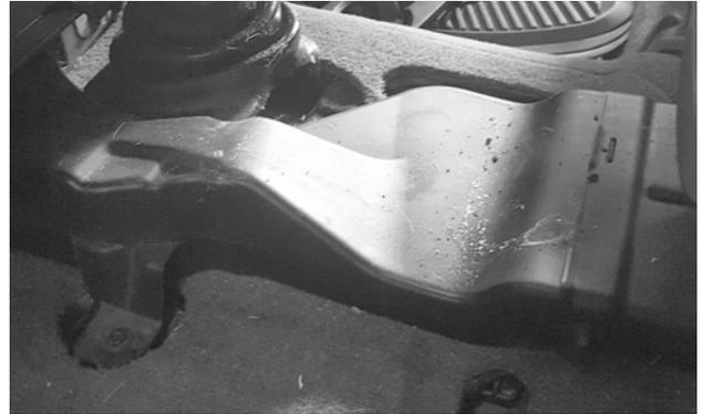
7. Remove the air conditioner / heater duct (if so equipped).
