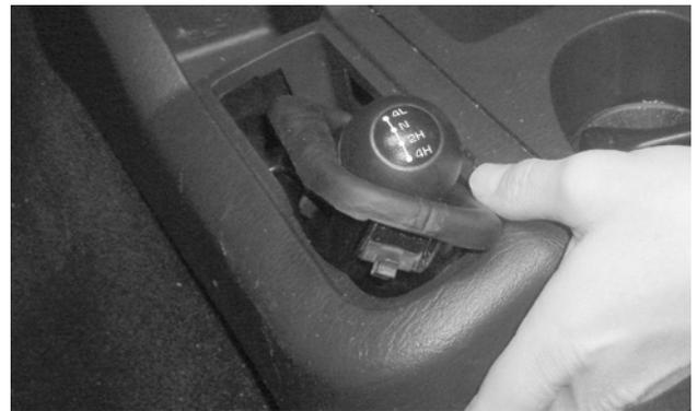
**NOTE:** For vehicles with a manual transfer case lever, tilt the boot frame slightly to fish it up through the opening.
