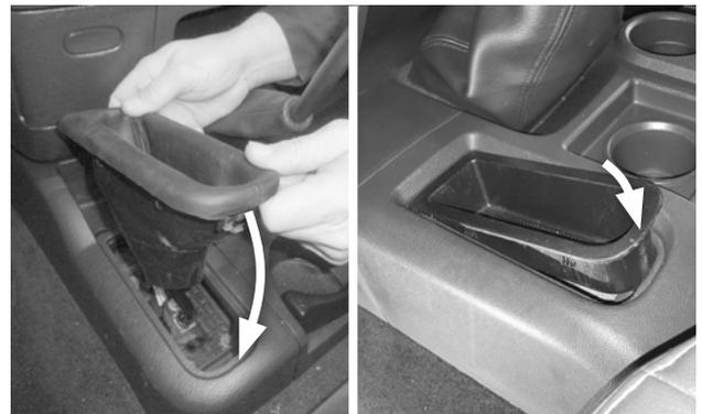
19. Reinstall the transfer case lever boot or the storage bin in the console rear half.
