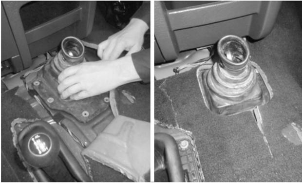
15. Reinstall the dust boot and screws, and return the carpeting to its place.
