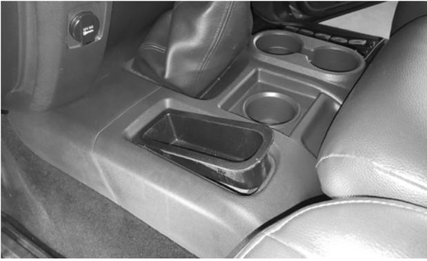
4. For vehicles with a storage bin (instead of a transfer case lever), remove the bin from the console.
