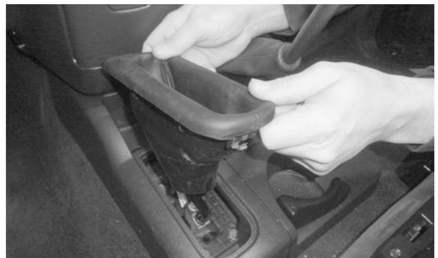
3. **For vehicles with a manual transfer case lever, move the lever to NEUTRAL, then separate the boot from the console and lift it clear, to access the console screw underneath.**
