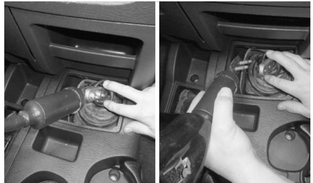
2. **At the bottom of the shift lever, pull the dust boot down** to expose the 2 nuts. Remove the nuts and the lever.
